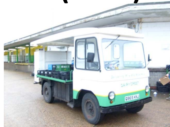
Milk Float, Smith Delivery Vehicles 75 mph; 65miles – Pb-Acid
