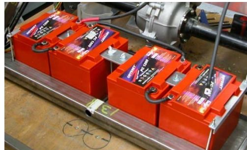
1.5 kWh Pb acid battery pack
