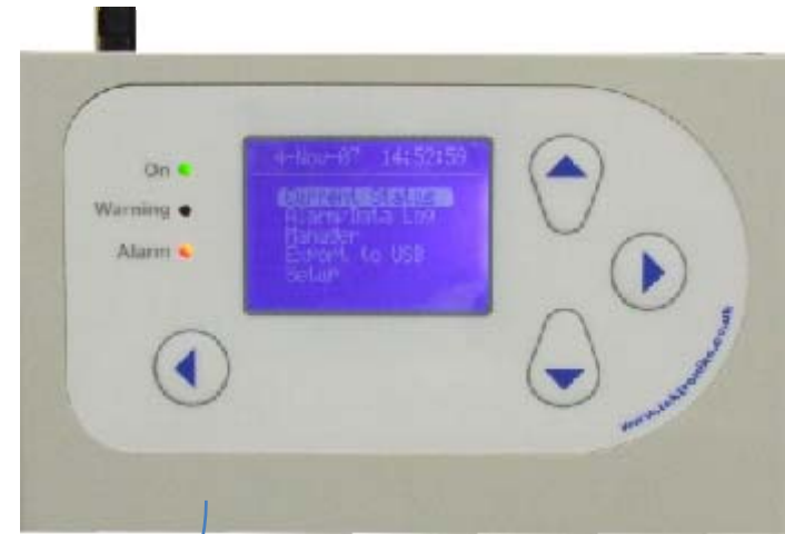
Wireless data logger
